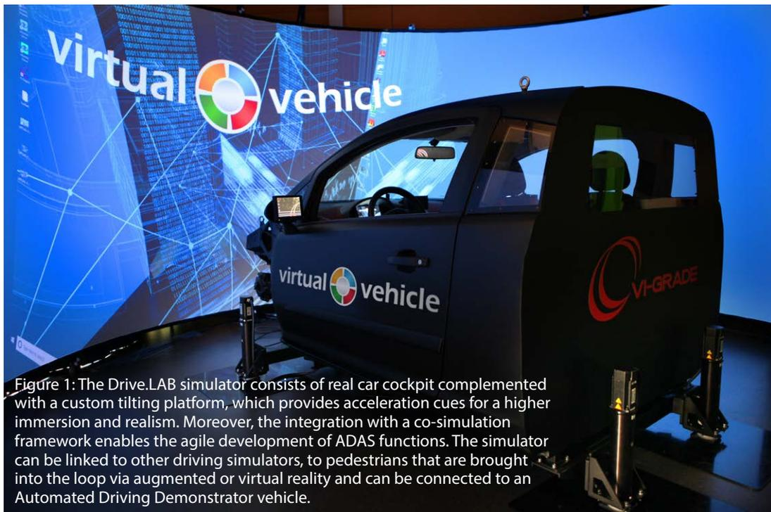
Figure 1: The Drive.LAB simulator consists of real car cockpit complemented with a custom tilting platform, which provides acceleration cues for a higher immersion and realism. Moreover, the integration with a co-simulation framework enables the agile development of ADAS functions. The simulator can be linked to other driving simulators, to pedestrians that are brought into the loop via augmented or virtual reality and can be connected to an Automated Driving Demonstrator vehicle.
